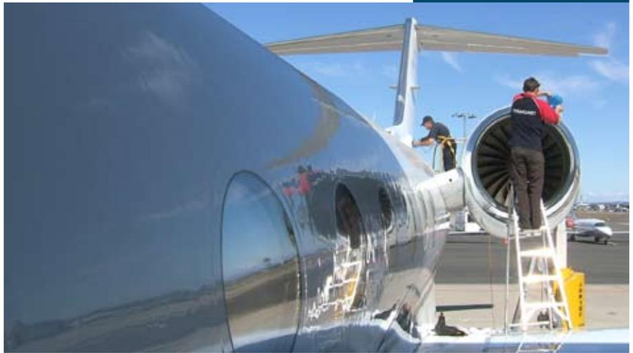
A Gulfstream IV has its paint treated using the Permagard protection system at Sydney Airport. Four people will take a combined 24 hours to complete the preservation. (Permagard)
